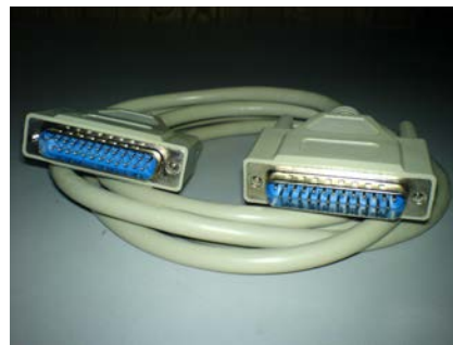
DB-25 pins Parallel Connector (One end to Parallel Port of PC, the other end to Parallel PB)
